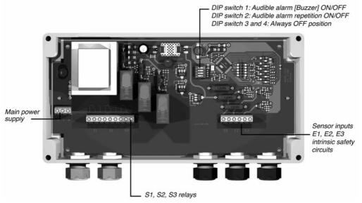
Do not connect the main power until the end of wiring
