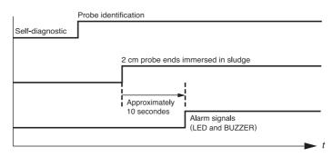
the test could be completed with the probe outside the separator and totaly immersed in water. after the auto diagnostic sequence, the control unit recognized the sludge probe and will:
