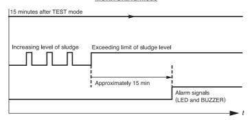
When you immersed the probe in water inside the separator, 15 min are necessary for the OilMatic Pro unit to validate the system conditions.
